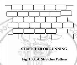
1504.11.1 By and large, this pattern is the same as adopted for brick paving. Paving shall commence and progress from one starting line only. Wherever possible, paving shall commence adjacent to or against edge restraint.
